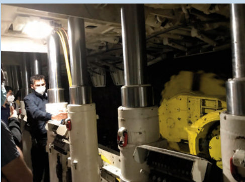
Below: Demonstration of a coal extraction machine with a self-advancing, hydraulically powered roof support.
